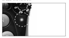
The LED indicator flashes every 4 seconds when the receiver is on and ready for use. The LED indicator will light up on both the transmitter and the receiver when the transmitter buttons are pressed. The LED color indicates battery life level.
