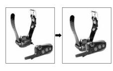
To turn the receiver on, place the red dot on the back of the handheld transmitter to the red dot on the receiver. Hold the two red dots together for a moment until the LED light on the receiver comes on.
