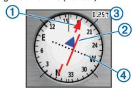
The course pointer ① indicates your relationship to the course line leading to the destination. The course deviation indicator (CDI) ② provides the indication of drift (right or left) from the course. The scale ③ refers to the distance between dots ④ on the course deviation indicator, which tell you how far off course you are.
