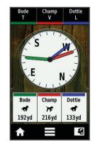
You can use the dog tracking compass to view the direction and distance to your dog. The dog tracking compass also shows the dog's status, such as running or on point (*Dog Status Icons*, page 5). The color of the pointer corresponds to the color of the dog track.
