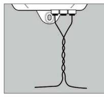
Splice the two ends of the twisted wire to each of the two ends of the fence wire. Drill a hole through the exterior wall or window/door sill or run the fence wire through an existing utility line hole. Connect the twisted fence wire to the transmitter, either wire to either terminal (wire ends must be stripped <sup>1</sup>/<sub>2</sub> inch),
