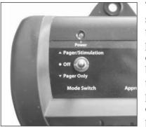
The On/Off & function selection switch has three functions. When the toggle switch is in the up position, the unit will give the dog a pager/vibration followed by stimulation correction. When the toggle switch is in the down position, only a pager/vibration occurs (no stimulation). The power is off when the toggle
