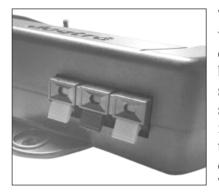
The easy-to-use push-release wire connectors let you instantly connect or disconnect the boundary wire leads. Wires should have the plastic coating stripped approximately a halfinch before being inserted into the red connectors on the bottom of the wall mount transmitter. The system comes with a ground
