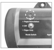
When the On/Off & function selection switch is either in the up or down position the On/ Off indicator light will be on, indicating that the power is on. When the switch is in the middle position the light goes off, indicating that the power is off. The indicator light stays on even if a fuse is blown.
