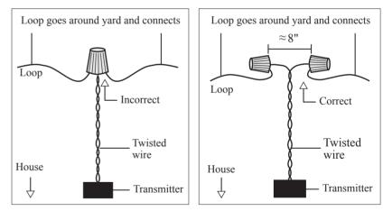
Incorrect Neutral Zone Wire Splicing Correct Neutral Zone Wire Splicing
