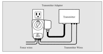
Plug the lightning protector into a grounded (3-wire) 120V AC outlet within five feet of where you want to locate the transmitter. Cut the e-fence wires near the protector and strip all four ends back <sup>1</sup>/<sub>4</sub> inch. Push the connector tab firmly away from yourself and the connector jaws will open. Push the stripped end of the wire into the connector.
