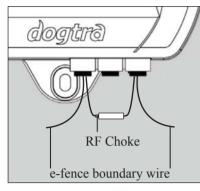
You will need a 100  $\mu$ H RF Choke and an AM radio tuned to AM530. Go to the wall mount transmitter and disconnect the two boundary wire leads from the RED connector tabs. In place of each boundary wire lead, connect one end of the RF Choke. Next, take the two boundary wire leads and reconnect them into the RED
