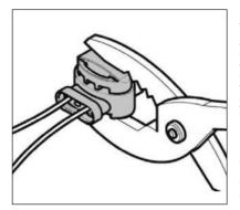
Do not use electrical tape, or soldered/twisted wire nuts in this type of connection as it will cause an intermittent signal or disarm the system. The waterproof splices included in the E-Fence 3500 system are designed to provide a sealed connection between the wires. The insulation on the boundary
