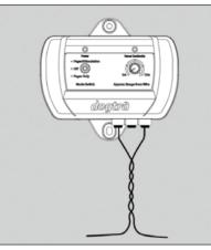
You must create a neutral zone from the fence transmitter to the beginning of the fence so the signals do not cross over to any existing utility wires. Start by twisting the two pieces of fence wire so they are braided from the beginning of the neutral zone area to the end. Braiding the two wires will interrupt the signal of the buried fence, thus creating an area for your dog to cross
