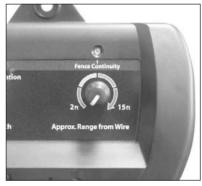
This knob controls the width of the signal field (the approximate distance from the boundary wire to the location where the receiver/ collar first activates). Turning the knob clockwise increases the field width, giving your dog a wider area before the activation begins. Turning it counter-clockwise decreases the signal field, thus
