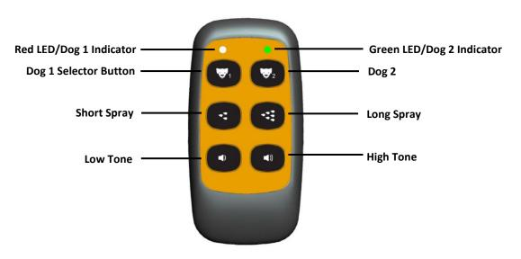
**Red LED Indicater:** When pressing Short Spray/Long Spray/Low one/High Tone button, if the Red LED flashes once, it means Dog 1 has been selected. The LED light will also flashes red in every few seconds to indicate the battery in Transmitter is low.
